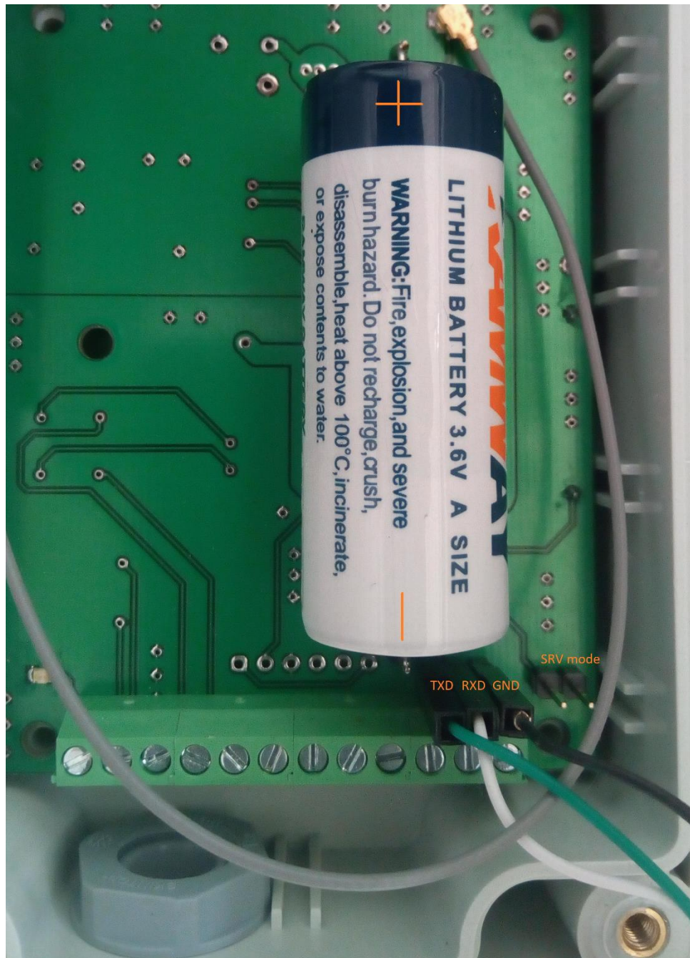
Figure 1 UART & service mode pins in 2 channel data loggers (v.4.2)
